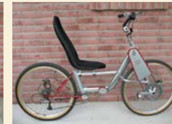
The aluminium-framed, rear-wheel drive bike, with crank axle passing through the front hub
