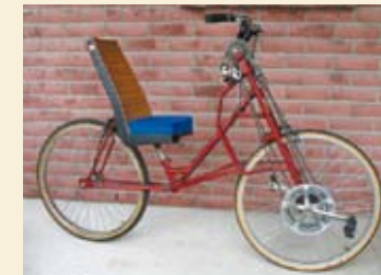
The first front wheel drive prototype, with a modified frame from a standard lady's bike.
